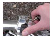
Over time the brake shoes which are fixed on the v-brake wear out causing a wider gap between the brakes and the wheel rim. This will be indicated in the leeway of the brake when applied. The left lever controls the rear brake and the right lever controls the front brake. You may also find as cables stretch the brake shoe on one arm will be moving more than the other. This will affect the safety of braking so will also need to be adjusted.
